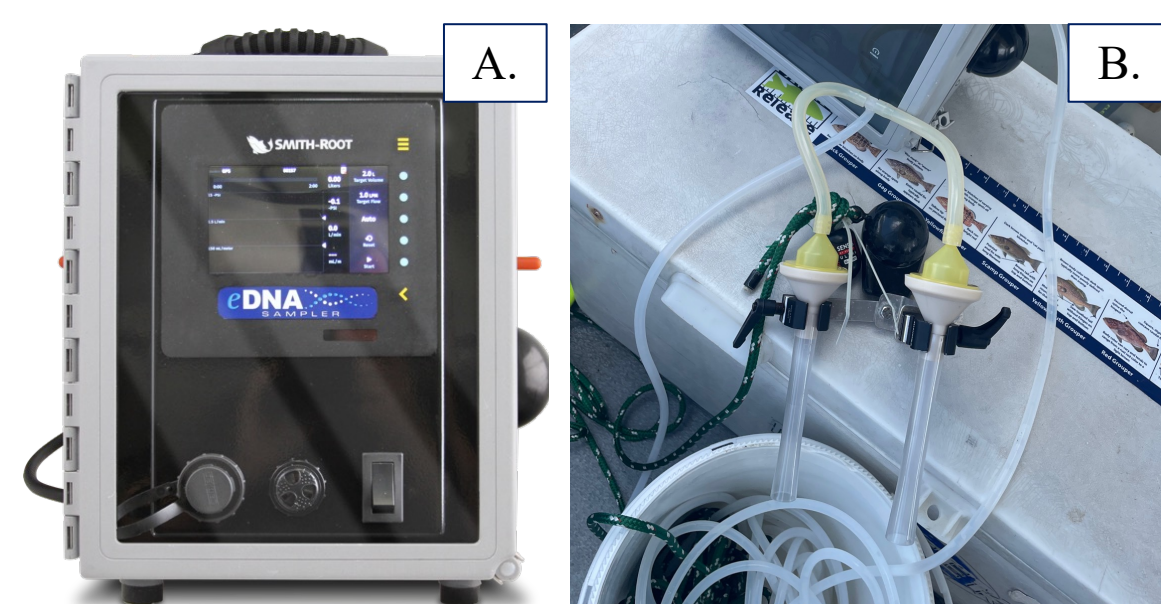
Figure 6. eDNA collection methods A) Smith Root eDNA water sampler and B) Two filter water collection method
