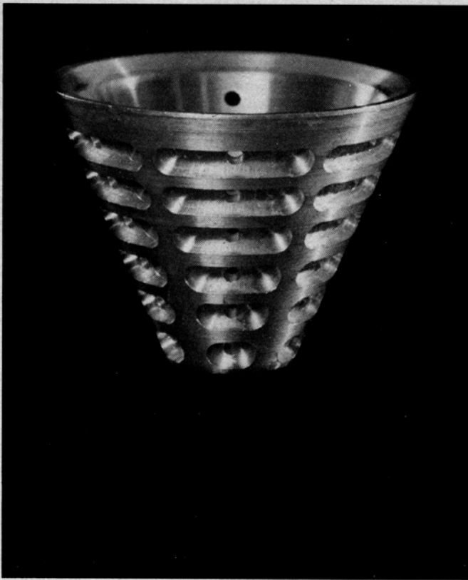
MODEL OF AN ARCHAEOCYATHID was made out of aluminum by William L. Balsam and the author at Duke University to enable them to test whether the animal was the right shape to take advantage of induced flow. In the assembled model the cone at the left
